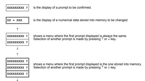
means pressing  $\mbox{\bf ENT}$  key to confirm a prompt or numerical data (changed or not).
