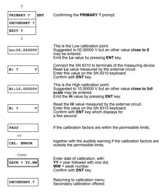
N.B: The primary calibration is performed on keyboard by entering one low point (Lo) and one high point (Hi). But using the IEEE-488 and RS 232 interfaces performs it in three points (see § 5.12.3.8).
