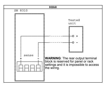
With the 2-wire configuration, voltage present on SENSE terminals of the SN 8310 is that programmed. Select the connection wires  $\frac{1}{2}$ according to the specifications of the tested unit.
