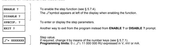
N.B: Display of \_\_=\*.XXXXXX indicates that recall of a step value stored in memory is not compatible with the selected range.
