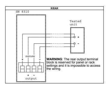
Avoid any stray e.m.f and minimize the resistance of the connection wires to the sense terminals.
